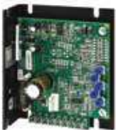
WPM Chassis Control (12 or 24 V models)
