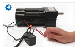
Connect the red wire from the motor to the other lead of the capacitor (Figures 4 and 5).
