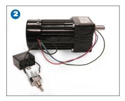
Connect the black motor lead to one lead of the capacitor. The capacitor is not labeled with polarities, so the connection may be made to either wire. Next, connect to the "throw" end of the single pole, double throw switch. The "throw ends" are normally the outer terminals of the switch (Figure 2).
