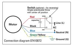
PART 1: Wiring without a direction switch Identify the wire colors and confirm that the gearmotor or motor is a 3-wire reversible PSC model. Bodine stock motors have red, black, and blue motor leads and a green-yellow ground lead.
