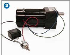
Connect the red motor lead to the other lead of the capacitor. Next, connect to the other "throw" end of the switch (i.e. the other outer terminal) (Figure 3).
