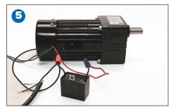
The capacitor must be permanently wired to the motor leads. Permanent split capacitor motors require a capacitor during start and while running.
