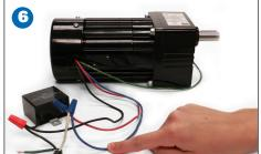
Connect the other side of the AC line. Connect the blue motor lead to the other lead of the AC line cord. Again, the connection may be made to either side (i.e. hot or neutral) (Figure 6).
