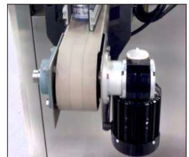
Conveyor with a Bodine Pacesetter 3-phase, AC inverter duty, hollow shaft gearmotor
