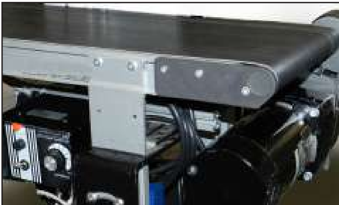
Belt conveyor with a Bodine 42A-FX gearmotor and WPM speed control
