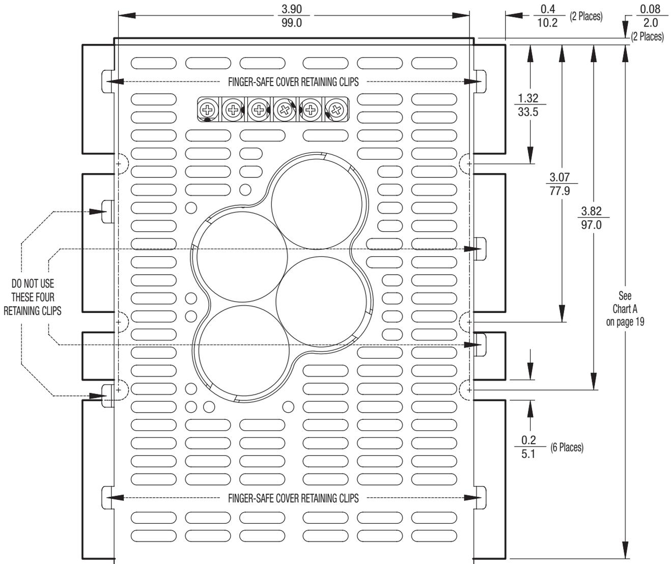
**FIGURE 3B – MODEL 2987 MECHANICAL SPECIFICATIONS (INCHES/MM)**
