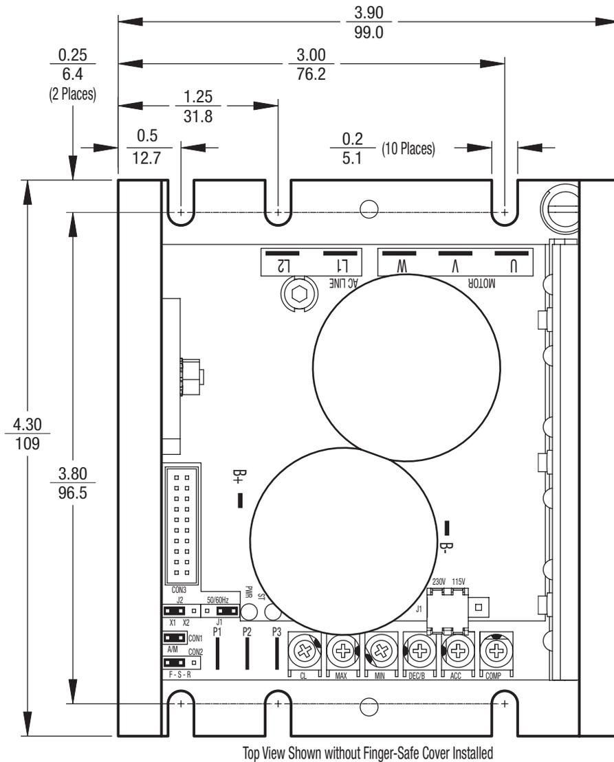
**FIGURE 2B – MODELS 2982, 2983, 2984 MECHANICAL SPECIFICATIONS
